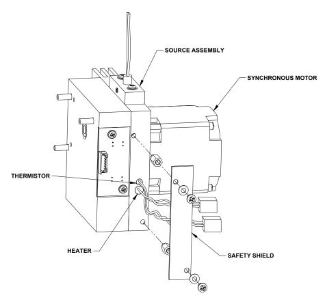
Figure 12-15: Opening the GFC Wheel Housing
